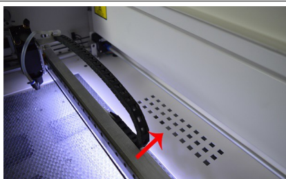
(1) Extraction vent and general cutting area.
