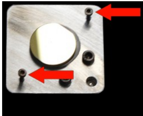
A 1.5mm Allen key can be used for mirror adjustment.
