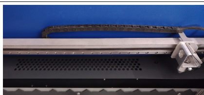
(1) Extraction vent and general cutting area.
